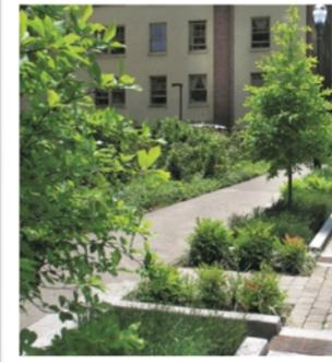
Stormwater planters (left) manage flow from impervious surfaces, allowing stormwater to infiltrate into the ground instead of the sewer system. The vegetation also filters pollution and reduces temperature.
