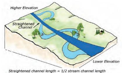
Straightened channel slope = 2 times stream channel slope
