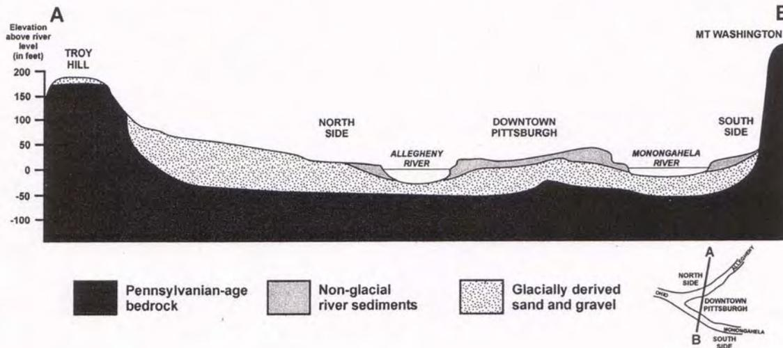
**Figure 2-4.** Cross section of Pittsburgh, showing the composition of the current river system. Taken from John Harper’s Geologic History of the Pittsburgh Area, DCNR.
