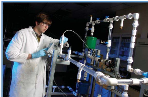
Experimental pipe loop system for evaluation of real times chlorine sensors. Dr. Damian Helbling is adjusting the sensor calibration. (Photo Courtesy Carnegie Mellon University)
