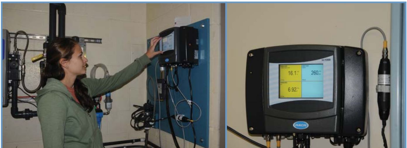
Water Quality Sensor Panel at two River Alert Information (RAIN) Sites. On left, Jess Wilson, graduate student at Carnegie Mellon University, reads the sensor values. (Photo Credit: Sandra Karcher.) ( www.3rain.org )
