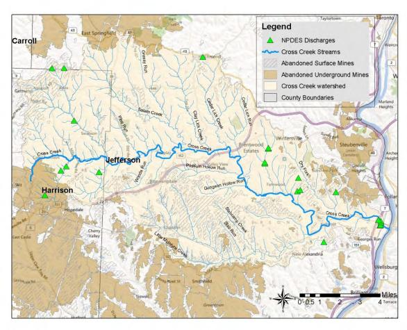
Figure 4. Abandoned underground and surface mines as well as NPDES permitted outfalls in the Cross Creek watershed (Jefferson and Harrison Counties).
