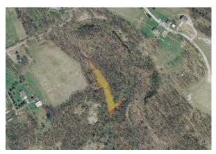
Figure 9. Aerial photograph of a pond located on the property of the Sisters of Reparation. The pond fills with iron laden mine water then discharges to a tributary to Dry Fork in the Cross Creek watershed.
